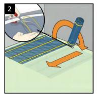
**Cut the mesh (not the cable)** Turn the mesh 180° and continue rolling
