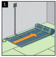
Roll out the mesh The mesh should be laid wire side down
