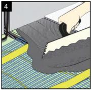
**Laying the tiles** Use a flexible tile adhesive to fix tiles straight over the heating
