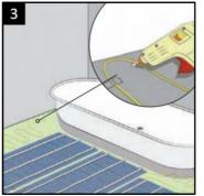
**Loose run for irregular areas** Remove the cable from the mesh, arrange and stick down
